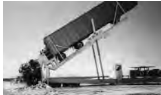
A trailer tipper emptying a transfer trailer at a waste disposal facility.
