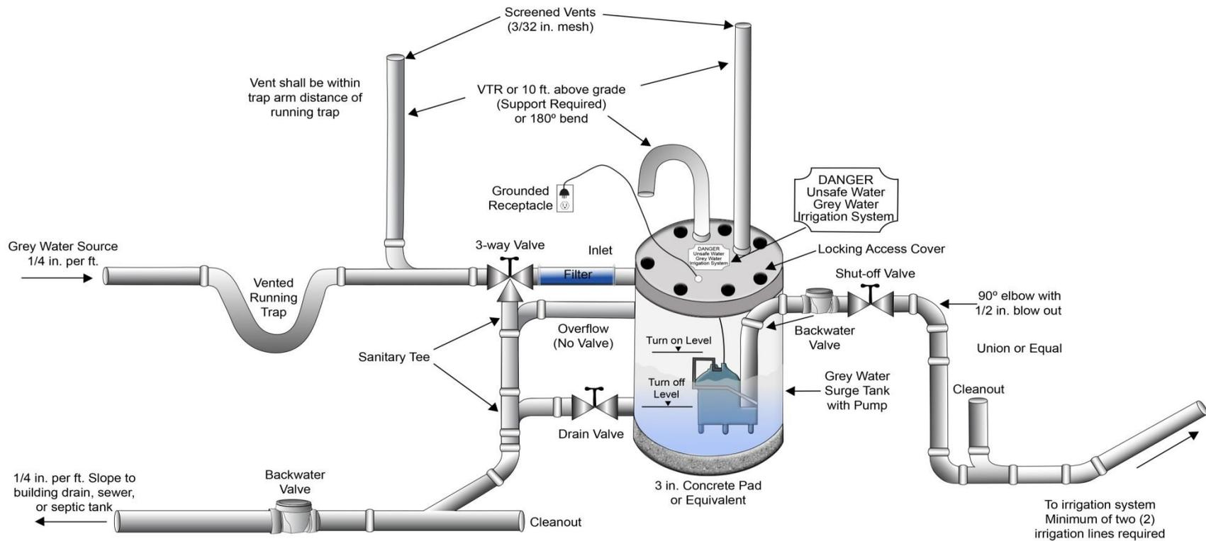
Figure 4-19. Grey water system (single-tank pumped).
