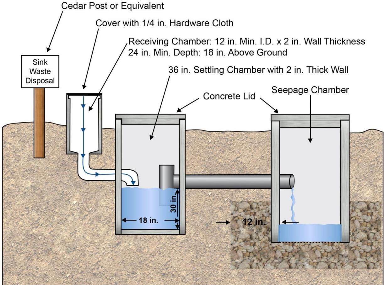
Figure 4-17. Cross section of grey water sump system.
