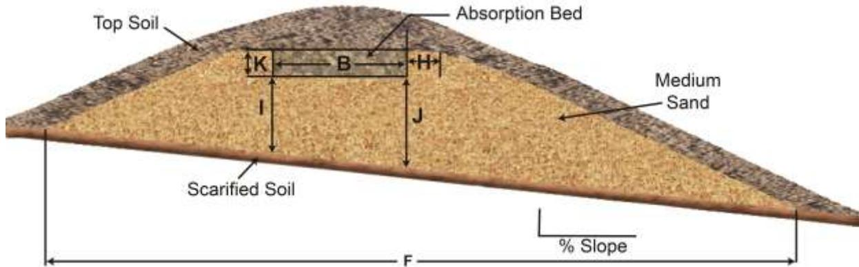
Figure 4-31. Design dimensions for use with the sand mound design checklist.
