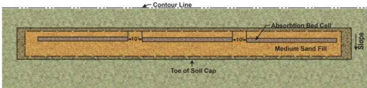
**Figure 4-29. Multiple absorption bed cells installed in one sand mound.**
