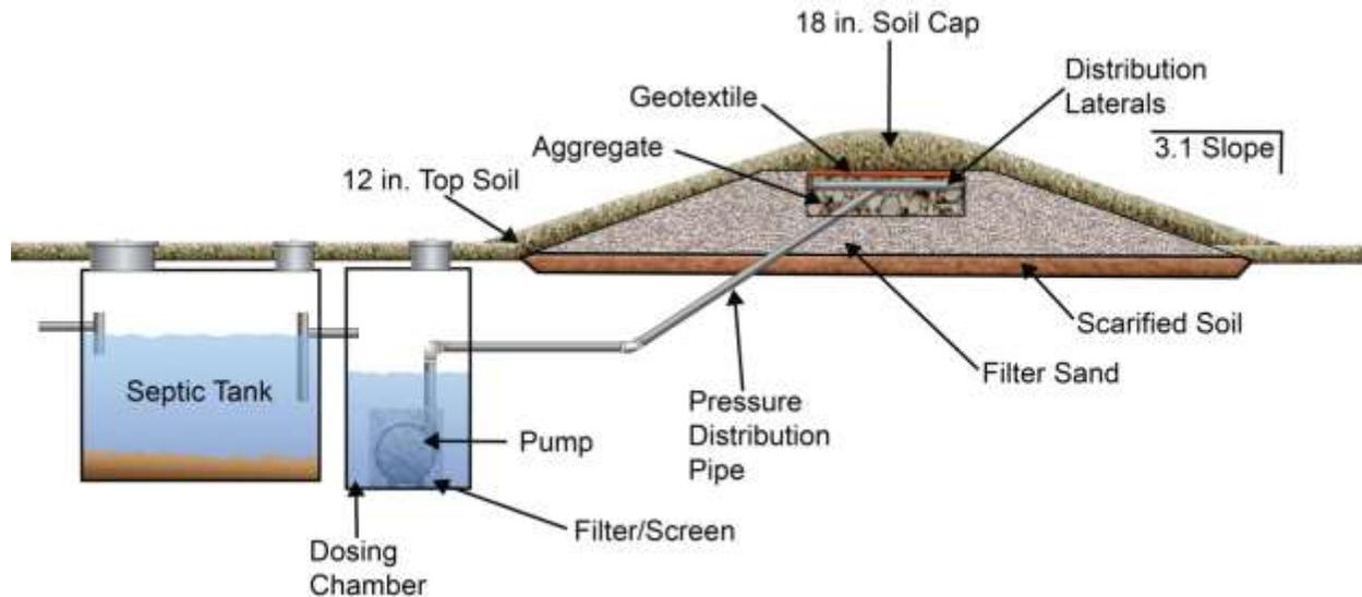
Figure 4-28. Cross sectional view of sand mound.
