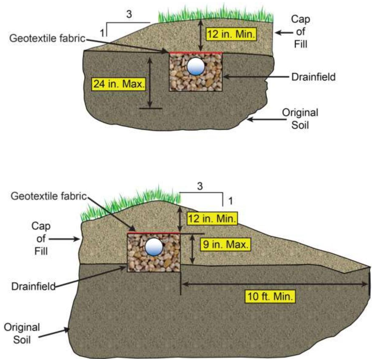
Figure 4-1. Cross-sectional view of a capping fill trench.
