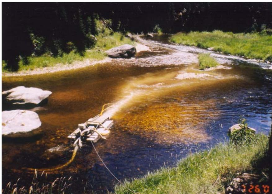
Figure 6. Sediment Plume from Suction Dredging.
