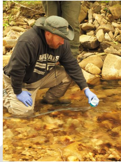
Collecting sample for eDNA analysis by filtering stream water.
