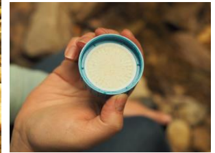
Collecting sample for eDNA analysis by filtering stream water.
