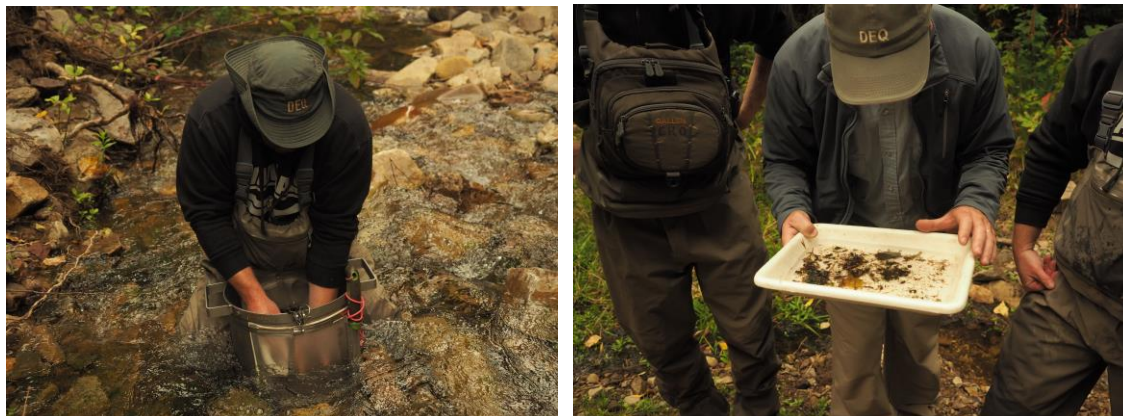
Collecting macroinvertebrates (bugs) samples using Hess sampler.
