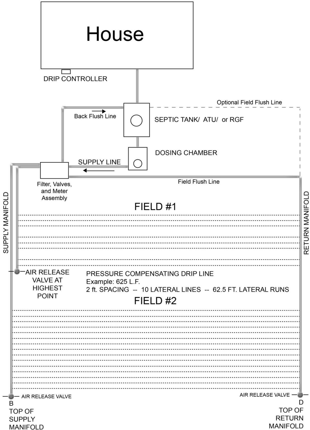
**Figure 4-7. Overhead view of typical drip distribution system.**
