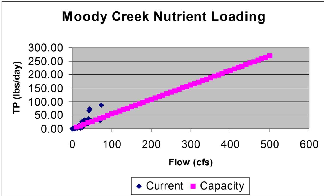
Figure 6. Current and Capacity Loading of Nitrogen in Moody Creek.
