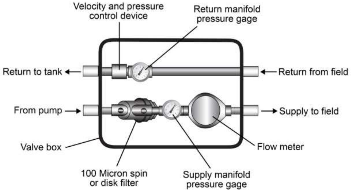
Figure 4-5. Overhead view of continuous flush system filter and meter assembly.
