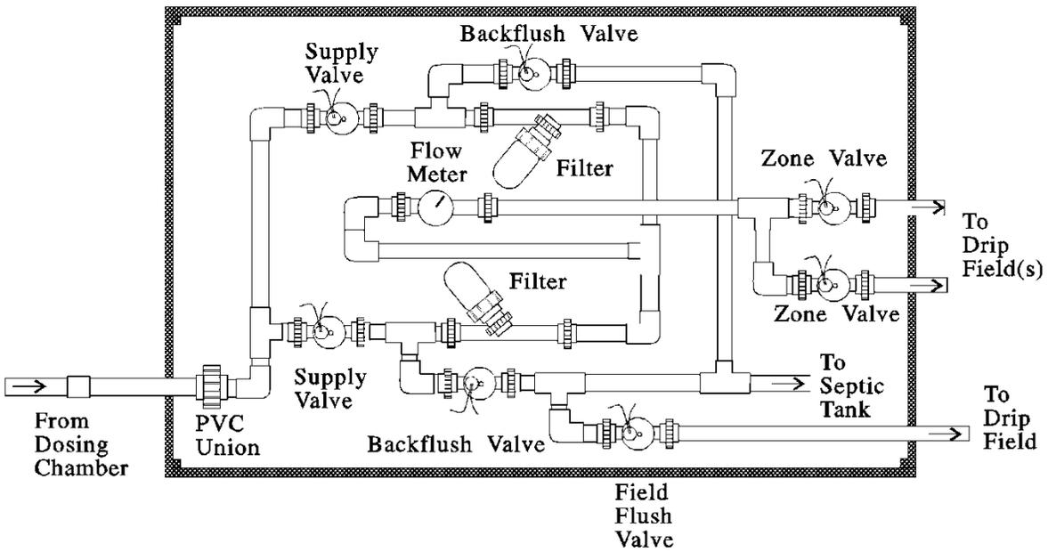
Figure 4-3. Overhead view of filter, valve, and meter assembly.
