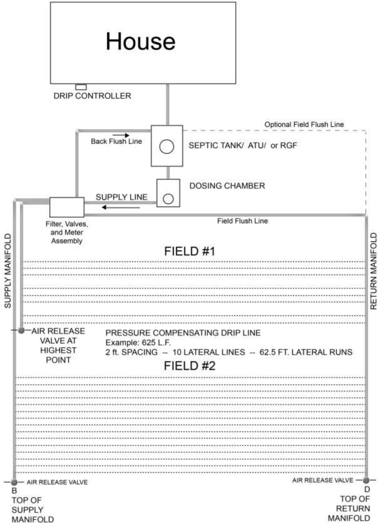
**Figure 4-2. Overhead view of typical drip distribution system.**
