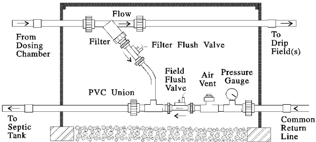
Figure 4-4. Cross-sectional view of typical filter, valve, and meter assembly.
