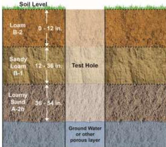
Figure 2-3. Test hole profile used in example 1.
