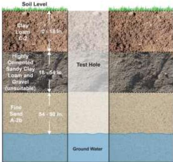
Figure 2-4. Test hole profile used in example 2.
