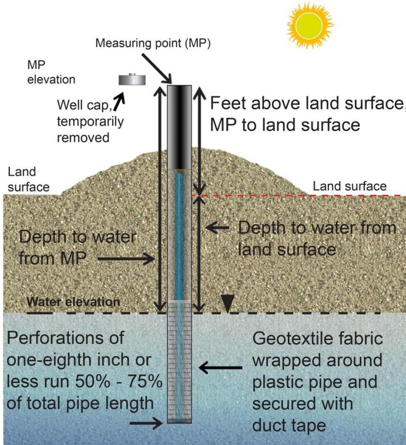
Figure 2-6. Temporary ground water monitoring well design.
