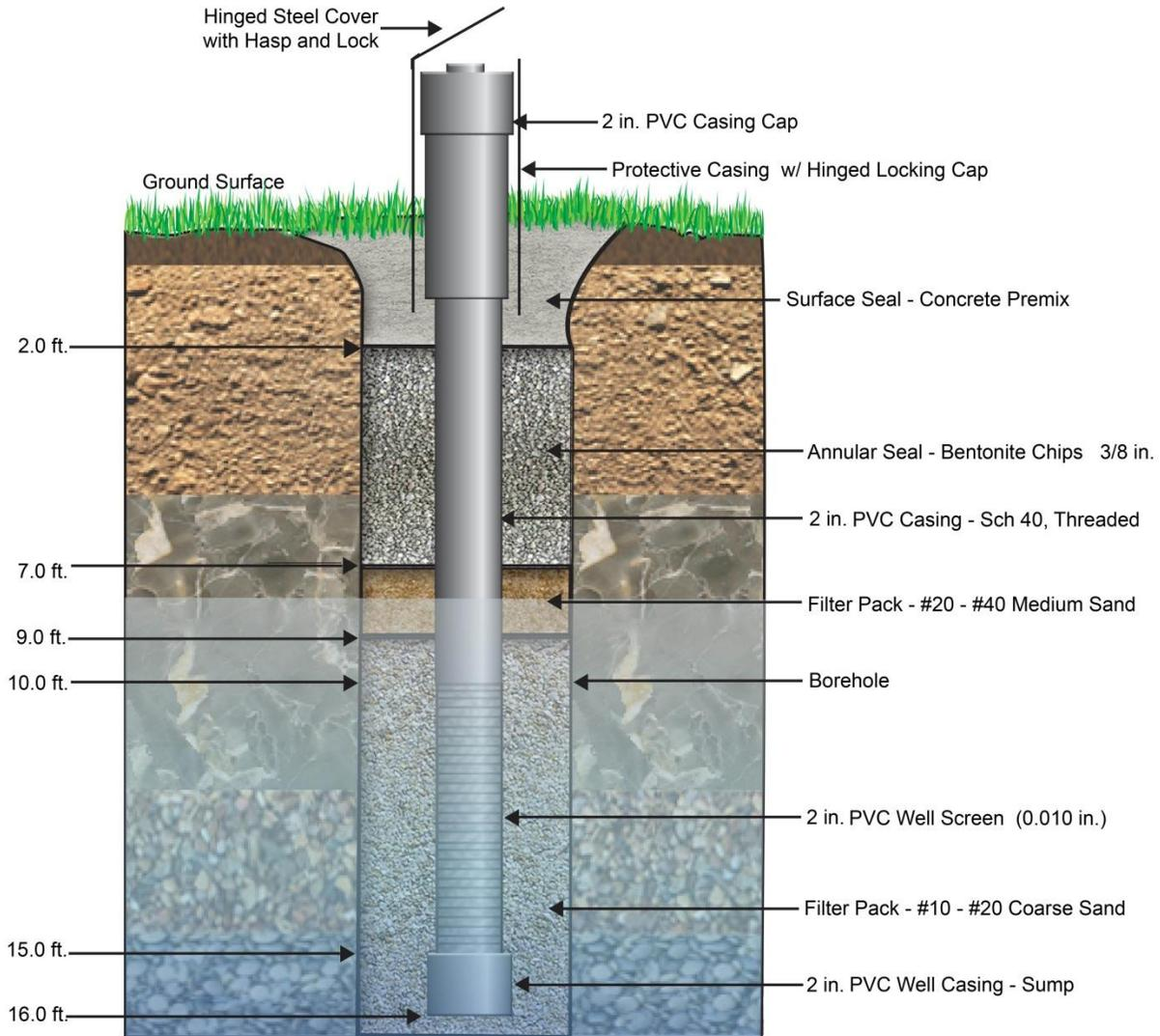
Figure 2-5. Permanent shallow ground water monitoring well design.
